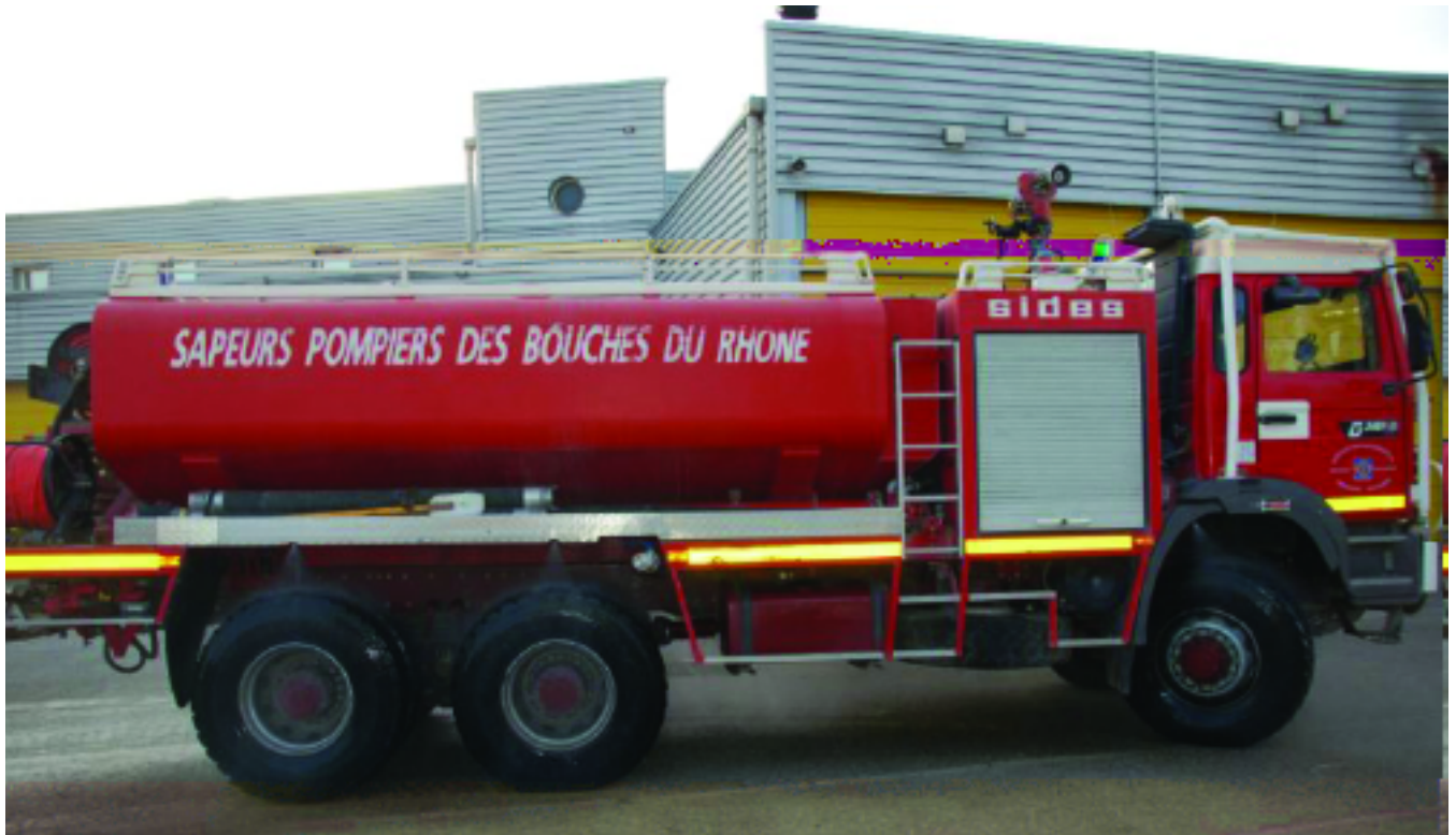
Newer construction, medium-duty steel unit. Note auto-protection wheel nozzles activating, white strip around door handle, white piping for external protection to the cab and tubing for spray nozzles to windows.
